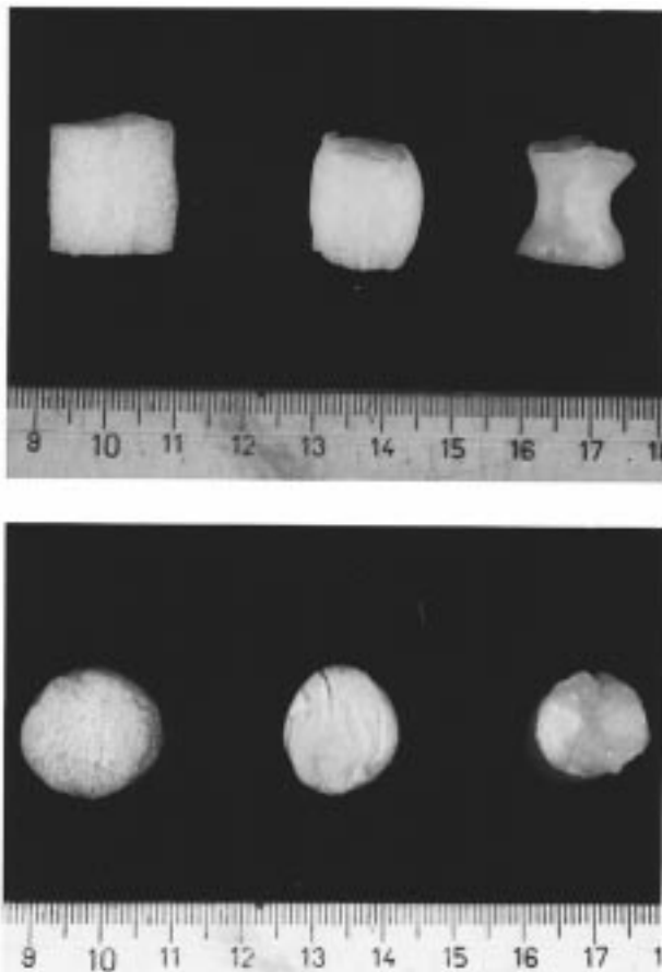
Figure 4. Photograph of dried cellular solids after immersion in 60 °Bx sucrose solution for 0, 4, and 48 h, from left to right. Upper panel shows front view; lower panel shows top view.
